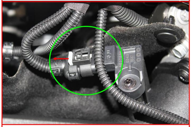
Please release Turbo-sensor 1, pull the grey clip of the connector back in the direction of the red arrow. Then pull down they grey clip to release the connector. Now put between the 2 tuning connectors
