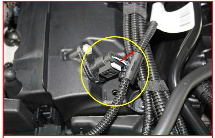
Please release the Camshaft sensor, pull the grey clip of the connector back in the direction of the red arrow. Then pull down they grey clip to release the connector.
