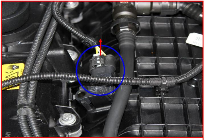
Please release Turbo-sensor 2, pull the grey clip of the connector back in the direction of the red arrow. Then pull down the grey clip to release the connector. Now put between the 2 tuning connectors.
