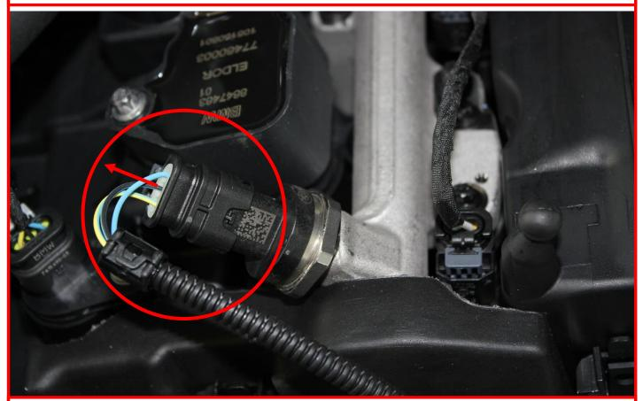
Please release Fuel pressure-sensor 1, pull the dark grey clip of the connector back in the direction of the red arrow. Then pull down they grey clip to release the connector. Now put between the 2 tuning connector.
